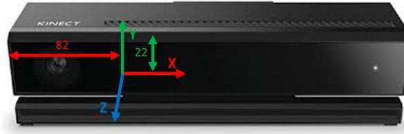
Figure 42: Location of the Kinect v2 reference frame. Values are in mm.
